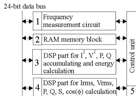
Fig. 2. DSP's block diagram
