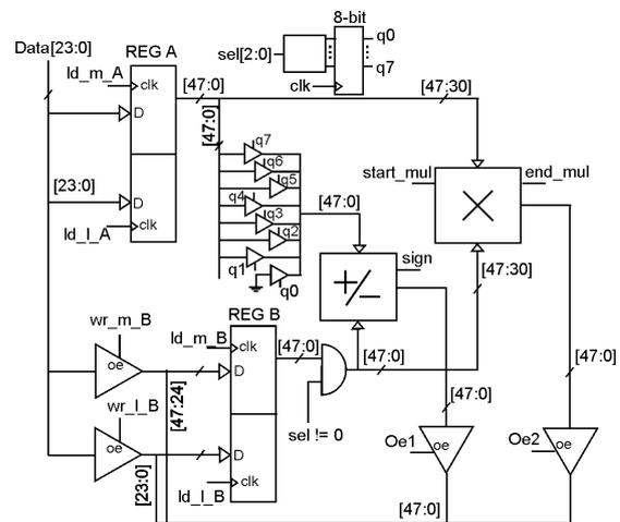
Figure 4 Part for  $I^2$ ,  $V^2$ , P, Q accumulating and energy calculation optimized for low-power by operand isolation and gating
