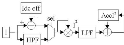
Fig.3. Data processing for current-square accumulation
